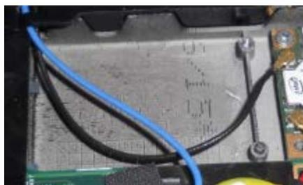
7. Take your MyDigitalSSD Super Cache 2 SSD and place it into the machine. It will only fit one way. Use the screw provided to secure it down. The SSD is now installed.
