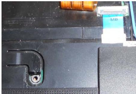
10. Next, reconnect the keyboard and close the lid. When putting the keyboard back in place, make sure to slide it under the lip.
