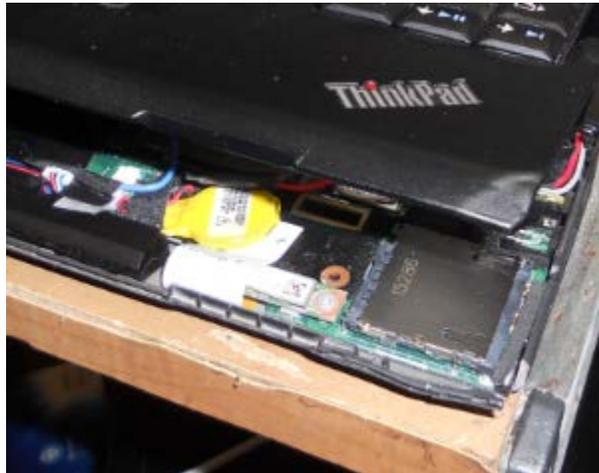
5. Reach in with the screw driver and flip the tab up to release the ribbon cable so you can open the top completely.
